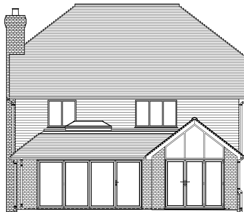
EXISTING REAR ELEVATION
